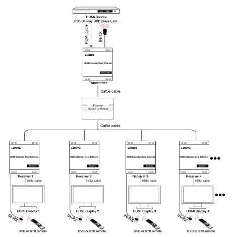
**W**<sub>Note</sub> Connect HDMI Transmitter port and Receiver ports to the Ethernet Switch
