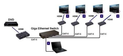
Figure 2. Demonstrate the 4K HDMI & USB Over IP Extender
