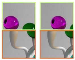
Adjust the vertical position of the video output, "Up/Down Shift", the selected monitor to adjust is shown with green outline.
