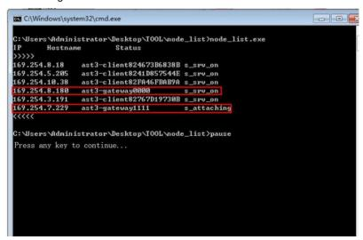
Remark: If the IP address with "Client", It's the IP address of the RX If the IP address with "Gateway", It's the IP address the TX.
