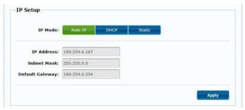
DHCP: use the DHCP of the external device such as the IP sharer to assign IP.
